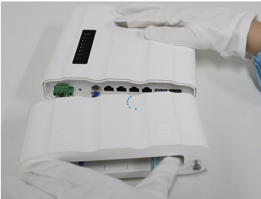
Figure 3-13 Connecting Cables to the Equipment (8)
