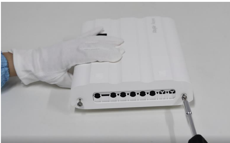
Figure3-4 Connecting Cables to the Equipment (1)
