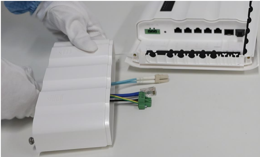
Figure 3-8 Connecting Cables to the Equipment (3)
